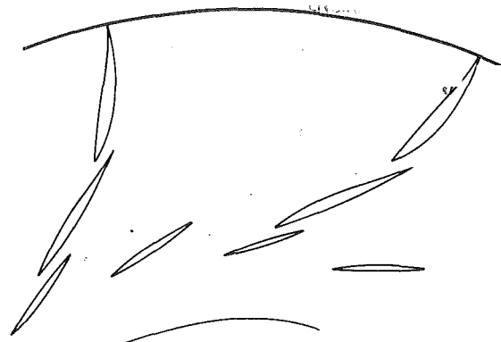
Fig. 6 Low-solidity cascade diffuser for automotive engine compressor
